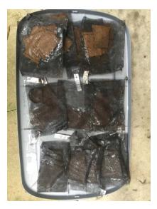
Figure 5. Mesh litter bags after washing of dirt sediments occurred.
