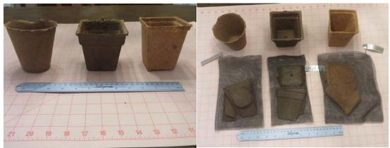
Figure 1. Cowpot, Fertilpot, and Coconut Coir pot containers placed in mesh bags designed from mesh fiberglass screen.
