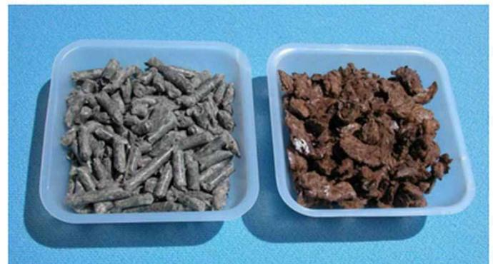
Figure 4. Examples of pelletized and processed and colored recycled newspaper that can be used as mulch.
